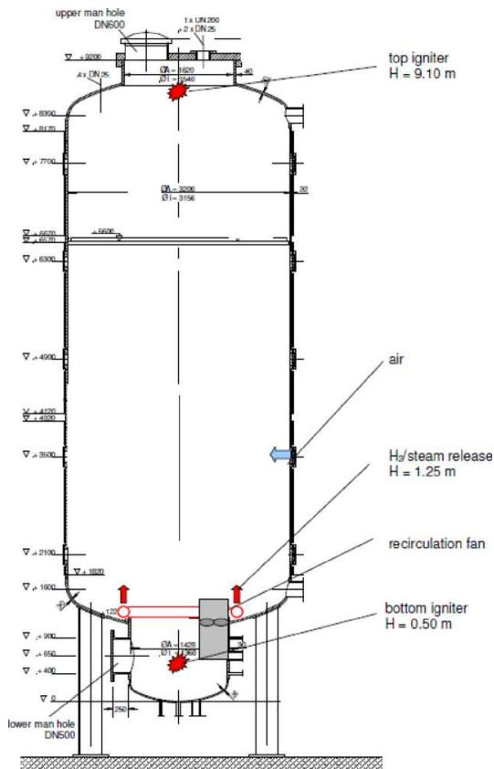
Figure 1 THAI test vessel configuration
