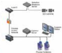
Typical Architecture Required for Experion PKS integration
